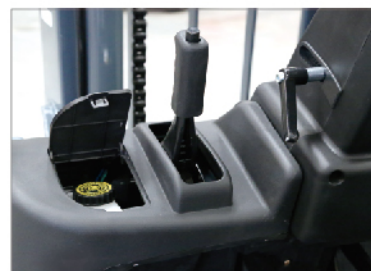
■ brake liquid reservoir
