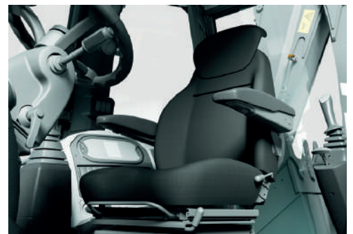
• Operator Seat with anti-fatigue with air-suspension for heavy-duty use over extended periods.
