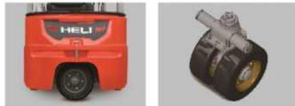
Be equipped with full hydraulic priority steering system, supply oil on demand, reduce vehicle energy consumption
