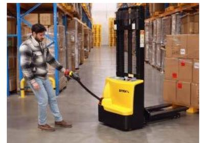
When truck is down, release the brake to move the unit manually.
