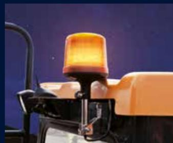
**Equipped with a new Type of LED Warning Light**
