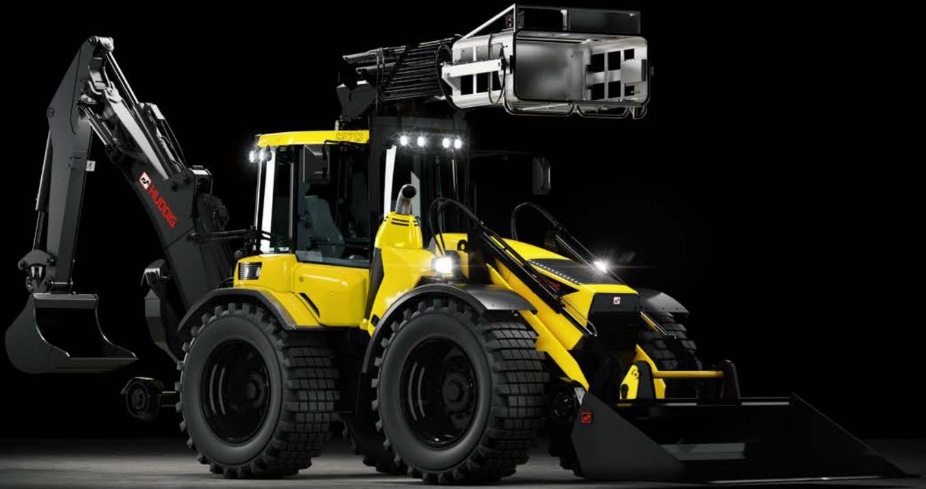
Huddig's RAIL machine can be equipped with powered or unpowered rail wheels
